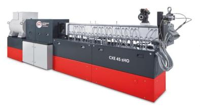
For the challenging processes of our customers we have implemented and developed our smart performance technology like our High Performance Elements as they are the segment and barrier screws for the gentle incorporation of glass fibers and/or thermosensitive flame
